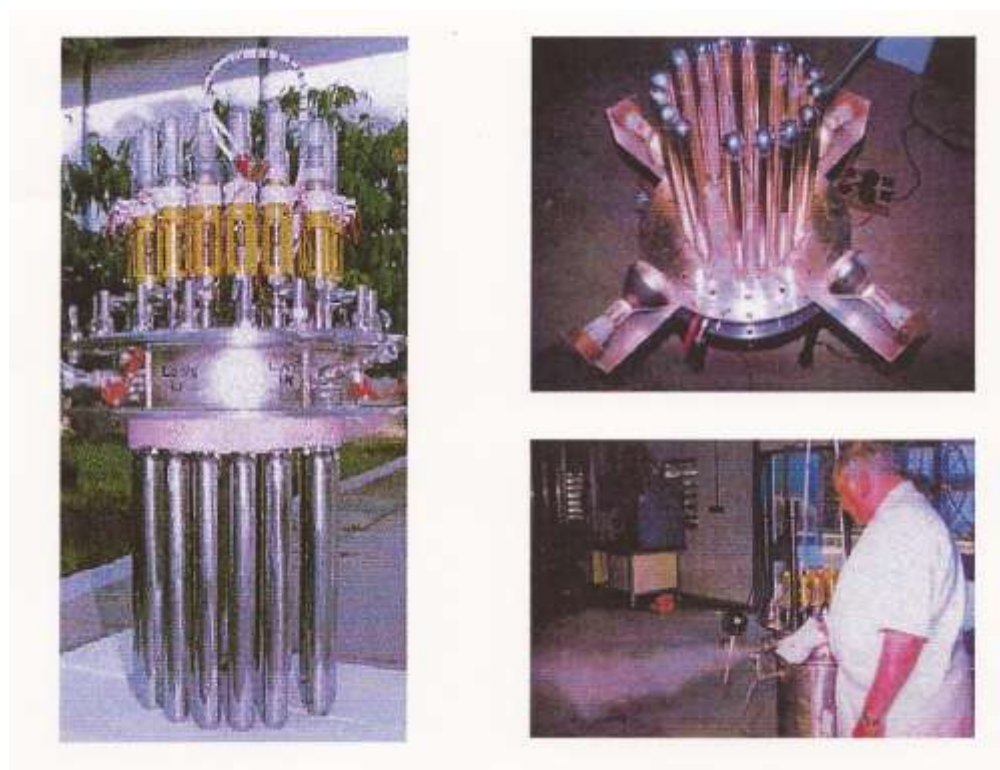
Figure 1: Evacuated and sterilised cryoprobes: Left : Assembled in a manifold ready for immersion in liquid Ne for launch. Top right : heat sterilisation under vacuum in an infrared setup at 140 degrees Celsius. Bottom right : steam sterilisation procedure.
